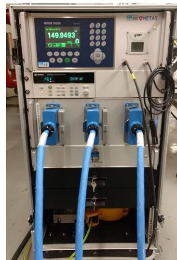
Figure 5: DAQ system with the various components (top to bottom): scale display, ambient conditions monitoring, multimeter and connection cables to the HFTS.
