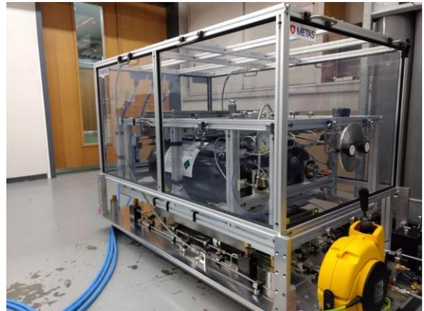
**Figure 2:** HFTS with housing, here partially closed. The open space between base plate and housing is 25 cm. The housing is not leak tight.
